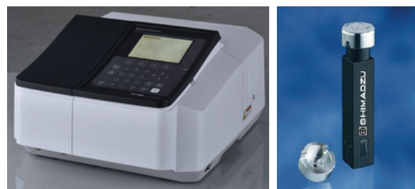
Fig. 1 紫外可視分光光度計 UV-1850 と TrayCell UV-1850 UV-Visible Spectrophotometer and TrayCell
