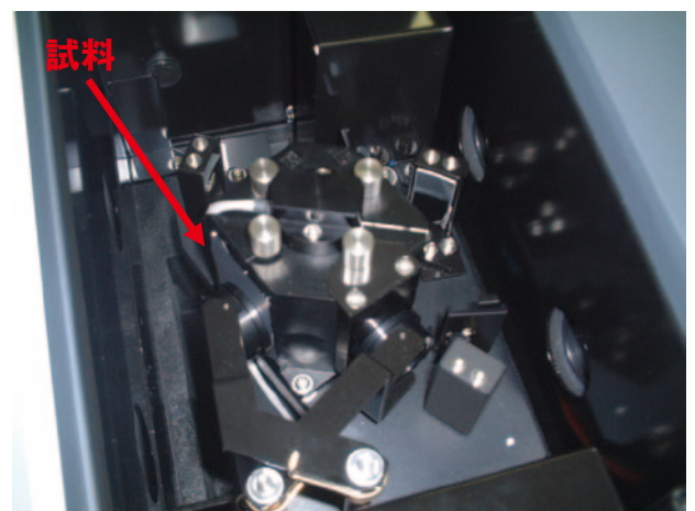
Fig. 3 積分球ISR-2600 Plus ISR-2600 Plus Integrating Sphere Attachment
