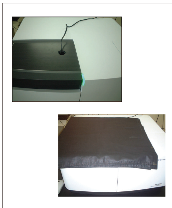
Fig. 3 暗幕を掛けて測定 Measured After Covering Sample Compartment with a Blackout Curtain
