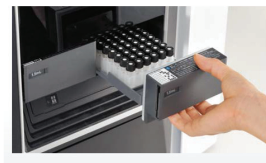
Fig. 2 ダイレクトアクセス機構 Direct Access Working for Each Sample Rack
