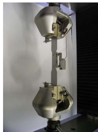
Fig.2 試験風景 Specimen and jigs for tensile test
