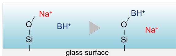
Figure 1 The proposed ion exchange mechanism between basic compounds and silanol groups
