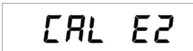
The image shows a rectangular digital display with the text "CAL E2" in a large, black, seven-segment font.
