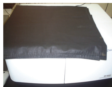
Fig. 3 暗幕を掛けて測定 Measured After Covering Sample Compartment with a Blackout Curtain
