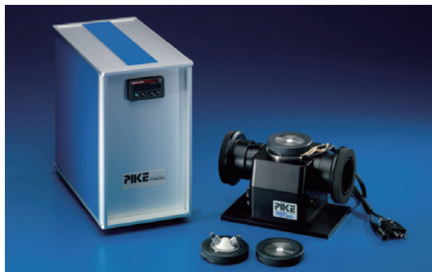
Fig. 1 PIKE製1回反射型全反射測定装置MIRacle A (加熱プレート) PIKE MIRacle A ATR Accessory with Optional Heated Crystal Plate
