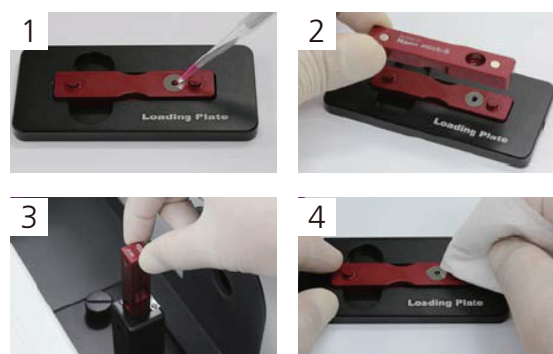
Fig. 3 Nano Stick の使い方 How to use Nano Stick
