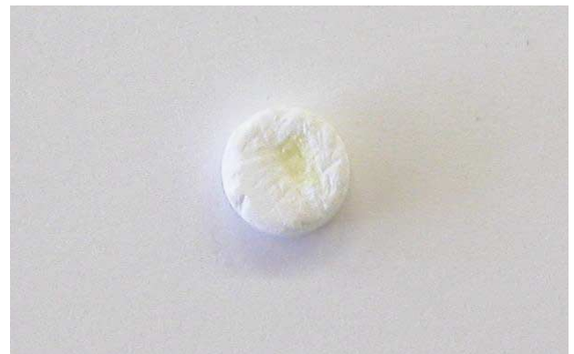
Fig.1 錠剤表面異物の実写真 Photograph of Contaminants on Tablet
