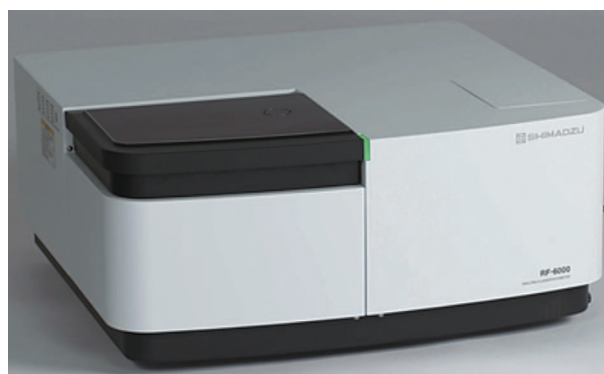
Fig. 1 分光蛍光光度計 RF-6000 RF-6000 Spectrofluorophotometer
