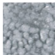
Fig.3 H 2 吹き付け後のNi Surface after H 2 blowing
