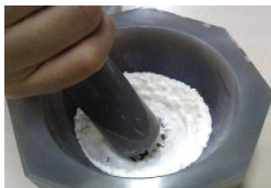
Fig. 2 粉碎・均一化 Homogenization by Pulverizing
