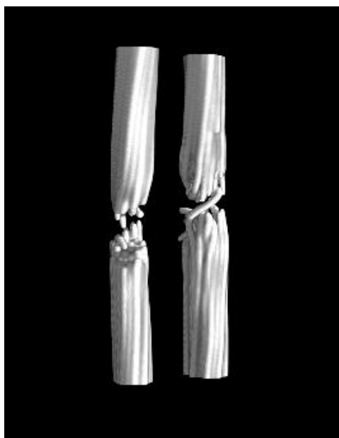
Fig.7-1 断線箇所の3次元画像 (SMX-1000-VCT) An example of 3-D image of disconnecting part.
