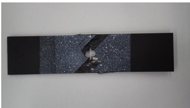
Fig. 6 破壊後の試験片 (正面) Specimens of After Failures (Front)
