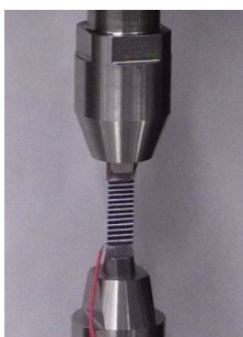
Fig. 1 CFRP 試験片と試験治具 Test Grips and Test Specimen
