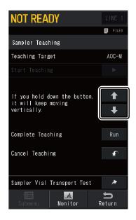
The arm keeps moving while a button is being pressed.
