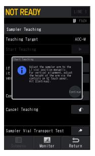
According to the value set in [Vial Type] on the [AOC Configuration] screen, the auto injector turnet turns and prepares for teaching.
