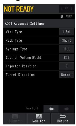
Set up the [Injector Position].
