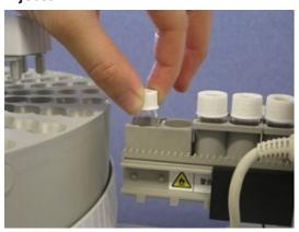
4 Set up the rack position of auto injector.
