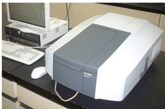
Fig. 2 積分球を装着した UV-2600 UV-2600 Mounting Integrating Sphere Attachment
