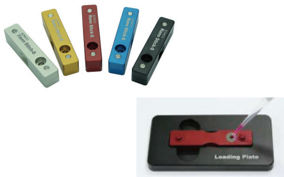
Fig. 1 Nano Stick の外観および試料滴下 Photograph of Nano Stick and Sample Pipetting
