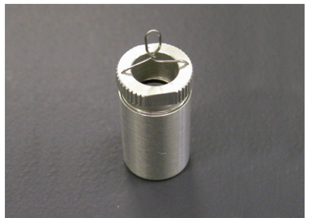
Fig. 2 透湿測定用試料セル Cell for Water Vapor Transmission
