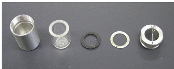
Fig. 3 透湿測定用試料セルの構成 Component of Cell for Water Vapor Transmission
