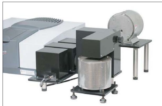
Fig.2 分光放射率測定システムの外観 Photograph of spectral emissivity measurement system
