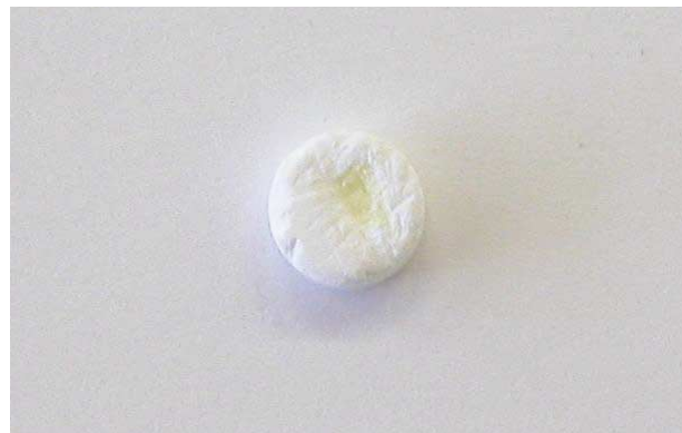
Fig.1 錠剤表面異物の実写真 Photograph of Contaminants on Tablet
